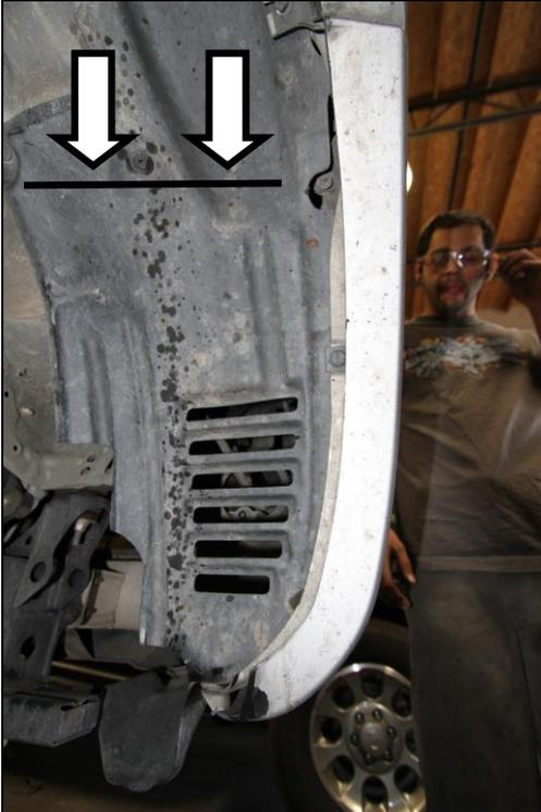
10.) To trim the inner fender plastic we recommend a box cutter for the cleanest and simplest method. If you would like further explanation, please see our video of the FJ bumper install that shows the cutting that is done of the inner fender lining. <https://www.youtube.com/watch?v=dF-B7inrDyU> at 4min 48seconds into the video it shows heating the box cutter which isn't necessary but does make the job easier.
