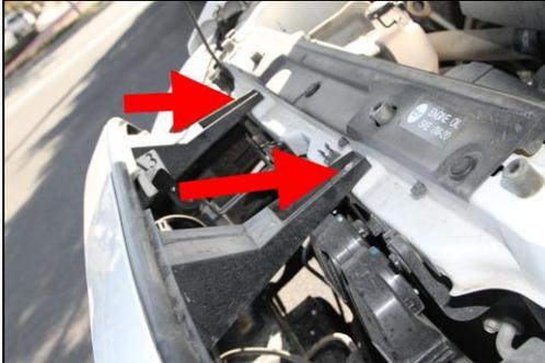
2.) Remove the two bolts securing the factory grill to the radiator support. These can be removed with a 10mm socket and 3/8in ratchet. We do not recommend using pneumatic or electric impacts as they may damage the hardware. Do not discard these bolts as you will re-use them. If you can't see the bolts in the picture, please refer to the e-mailed instructions as the pictures may be clearer to see. You can also find many pictures on line by Googling "2016 Tacoma grill removal"
