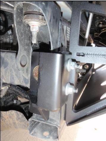
16.) Slide the brackets “**OVER THE BUMPER**” and the frame, clamping the bumper to the frame. **Some** tacoma’s will have plastic caps in the frame that will need to be removed so that the 1/2in bolts can easily pass through the frame. Put all the hardware in place secure it down but do not fully tighten so you can adjust the bumper to your liking. There should be two factory outter nuts preside shown here as well as two inner nuts (not shown) one on each side holding the bumper down.
