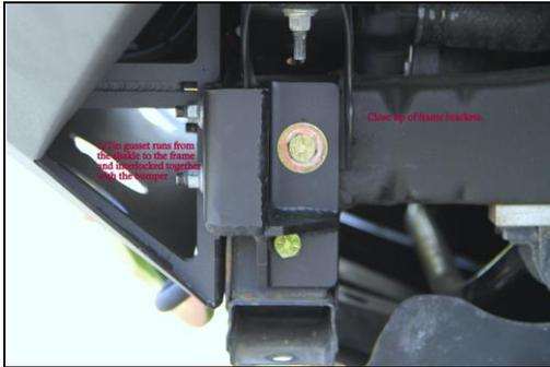
17.) Here is another shot of the bracket showing how the bracket clamps the bumper to the frame. Again you should have 6 total factory nuts holding the face of the bumper to the Tacoma frame. You will also have two 1/2in bolts that pass through the frame the opposing direction as shown here with the nuts and supplied washers in the order shown in step #15.
