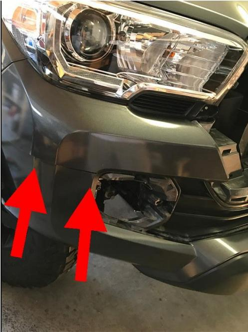
8.) Shown again is the line where the bumper has been cut. (not shown) we use a small cut off wheel to cut this portion of the bumper. You can also use a dermal or air saw as well. Shown also in the picture is the fog light removed which you don't have to remove, but if you wish too you can.
