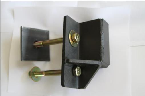
15.) with the bumper in place, locate these brackets. Note the order in which the bolts, washers and backing plate go on the frame and on the bumper.
