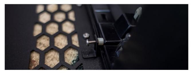
13) Locate the remaining six tabs at the bottom of the new Inner Grille. Using the **six (6)** ½" **Phillips stainless steel screws**, place in the remaining tabs and gently screw in until the plastic bites.
