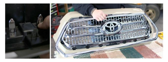
NOTE: These tabs are made of plastic and can break easily! Be gentle to prevent breaking.
