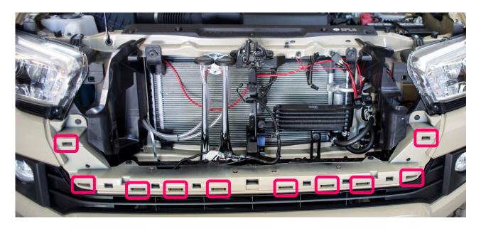
Insert the Front Bumper Unit beginning at the bottom and continuing up as all tabs fall into place.
