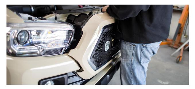
16) Once the Front Bumper Unit is sitting securely in place without any visible gaps, reattach the **two** (2) Phillips bolts on the middle legs and the **two** (2) black retainer clips near the headlights.
