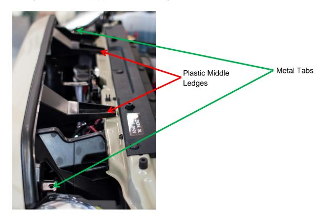
2) Locate the **two (2) black retainer clips** on the metal tabs. Insert the tip of a flathead screwdriver under the button lip of each clip and push the button up until the entire clip comes out.
