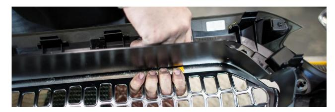
You should now have the unit separated into three parts: Bumper Faceplate, Outer Trim and Inner Grille.
