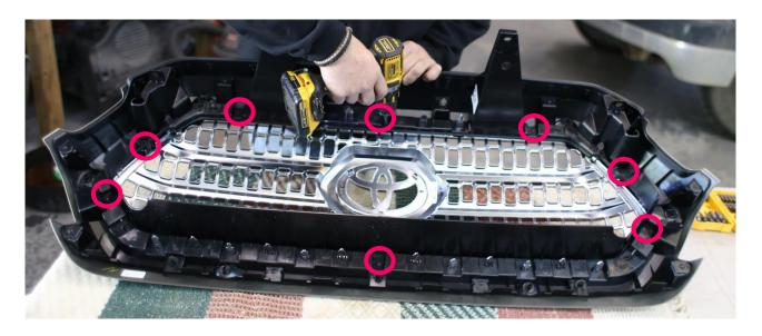
7) Gently squeeze in **the eight (8) silver tabs** that hold the Outer Trim, while lightly pulling on the outer trim with your other hand, to ease its release.
