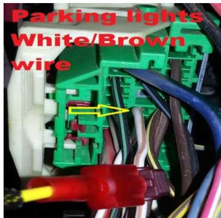
Figure 2. Parking light wire
