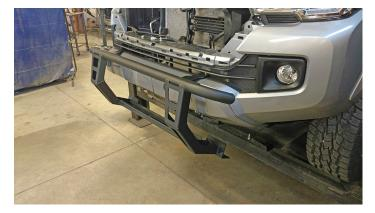
$\begin{array}{l} \textbf{11.} \text{ Swing the push bar up into place on the front cross member} \\ \text{and using the bolts that hold the little horns in, loosely thread} \\ \text{them in. now center the push bar and tighten these bolts down.} \\ \text{- Photo L} \end{array}$
