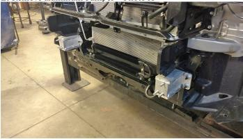
**3.** Slip mounting brackets over the bumper mounting bolts. – Photos B & C
