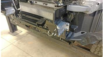
${f 4.}$  Slip bumper over the brackets and tighten down nuts. – Photo D
