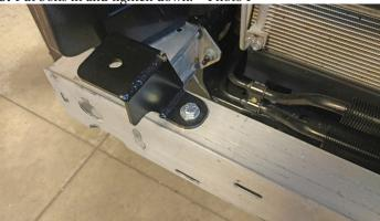
**7.** Bolt extension brackets on using  $3/8 \times 3/4$  hardware as shown just using the bolts. – Photo G
