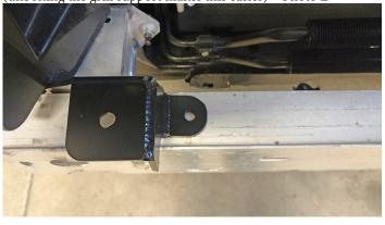
**6.** Put bolts in and tighten down. – Photo F
