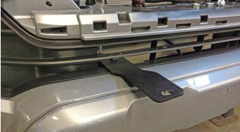
**10.** Hang the push bar on the mounts, line up holes and loosely tighten bolts.—Photo K
