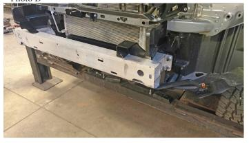
**5.** Drill out aluminum bumper to accept the 3/8" bolts (unbolting the grill support makes this easier) – Photo E
