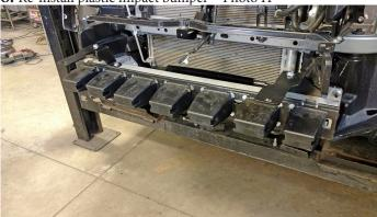
**9.** Install plastic bumper shell, be careful to slip push bar extension brackets through the widest openings in bumper grill
