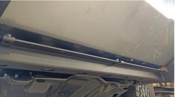
15. Install license plate on center plate and bolt center plate to push bar.
